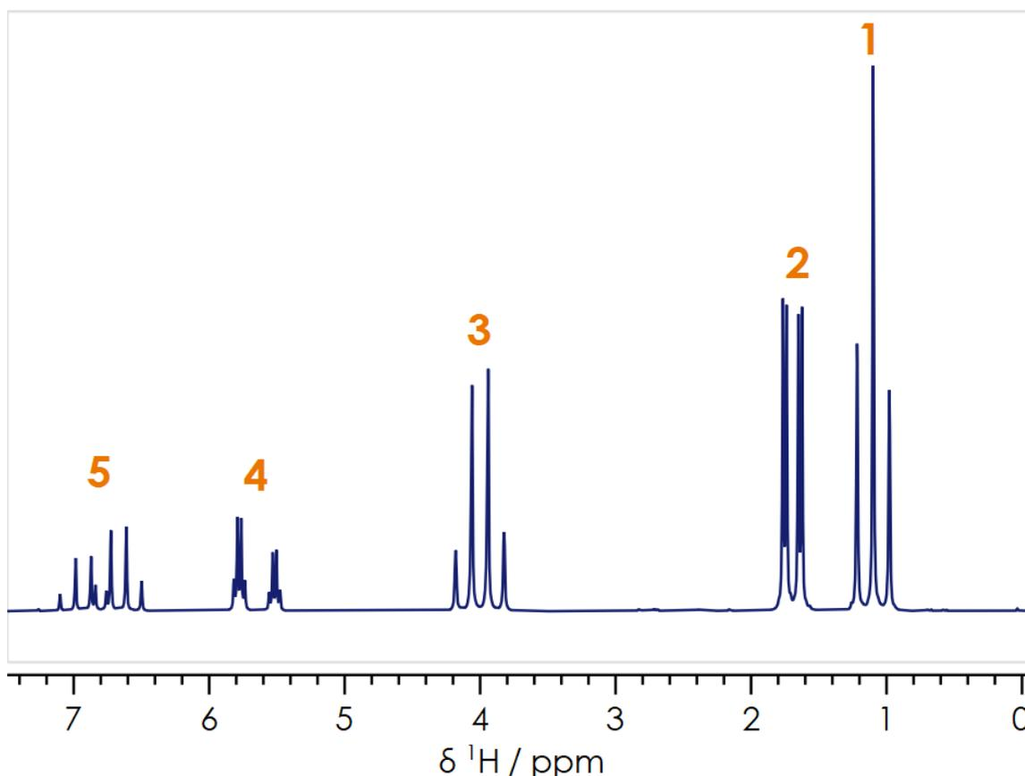
Figure 3:  $^1\text{H}$  spectrum of ethyl crotonate in  $\text{CDCl}_3$  acquired at 60 MHz
