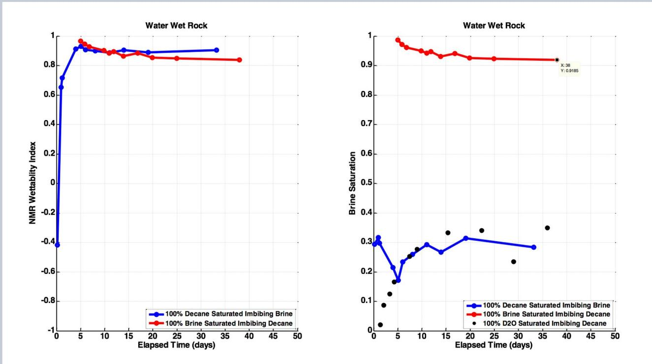
**Figure 4:** The results of the wettability analysis for twins 2-P1A and 2-P2 are shown. The left-hand panel shows the wettability as a function of imbibition time for both samples, while the right-hand panel shows the water saturation as a function of imbibition time for both samples. The black dots the water saturations as determined in a separate NMR measurement on a different 2P sample 100% D2O saturated imbibing decane.
