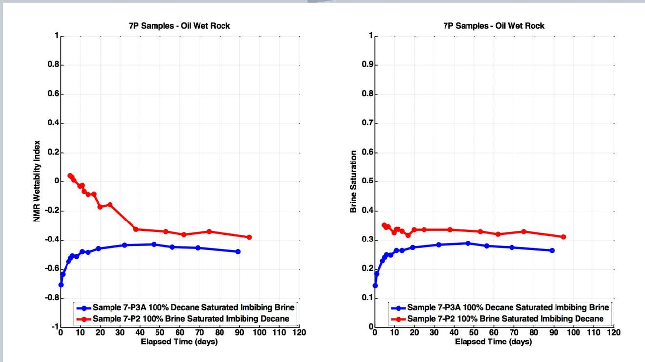
**Figure 5:** The results of the wettability analysis for twins 7-P3A and 7-P2 are shown. The left-hand panel shows the wettability as a function of imbibition time for both samples, while the right-hand panel shows the water saturation as a function of imbibition time for both samples.
