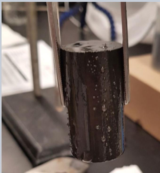
**Figure 1:** Water droplets seen on the surface of the sample after it was submerged in decane.
