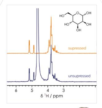
Shaped pulses and pulsed field gradients improve solvent suppression. Pulsed field gradients additionally measure self diffusion.
