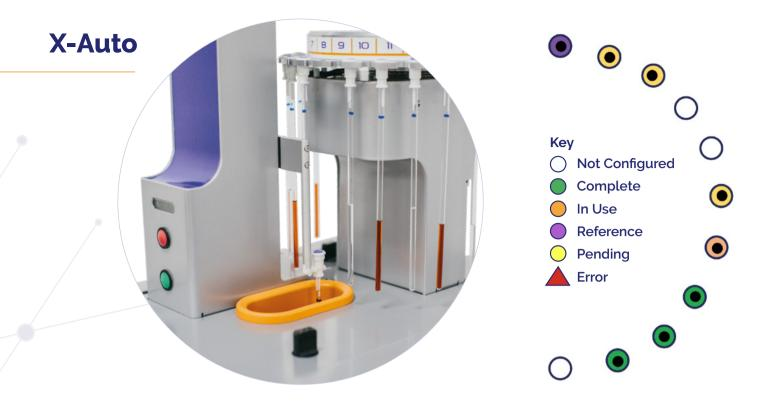
Fully automate data acquisition across 25 samples, all controlled from within the **SpinFlow** acquisition software. No need to stop to add new samples, just drop the sample in and set up your experiments. **X-Auto** provides you with the flexibility you need for your experiments - use different NMR tubes with lengths ≥20 cm, diameters ≤5 mm, and a range of specialist fittings.
