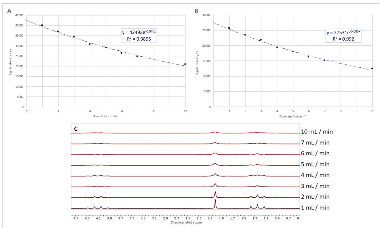
**Figure 2:** A – Signal intensity as a function of flow rate for the  $\text{CH}_3$  resonance of the ethyl group of ethyl ethanoate; A – Signal intensity as a function of flow rate for the  $\text{CH}_2$  resonance of the ethyl group of ethyl ethanoate; C –  $^1\text{H}$  NMR spectra of ethyl ethanoate collected at different flow rates
