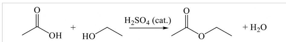
**Scheme 1:** Esterification of ethanol and ethanoic acid catalysed by sulphuric acid to produce ethyl ethanoate and water
