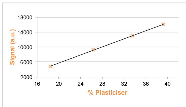
Figure 2: NMR calibration for plasticiser in PVC
