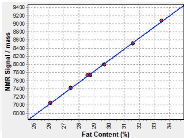
**Figure 1:** NMR calibration for Total Fat Content of **dark and milk chocolate** referenced against the IOCCC method. The correlation coefficient ( $R$ ) and standard deviation ( $\sigma$ ) are 0.999 and 0.07 respectively.
