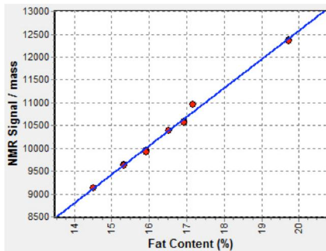
**Figure 2:** NMR calibration for Total Fat Content of **chocolate crumb** referenced against the IOCCC method. The correlation coefficient ( $R$ ) and standard deviation ( $\sigma$ ) are 0.997 and 0.12 respectively.
