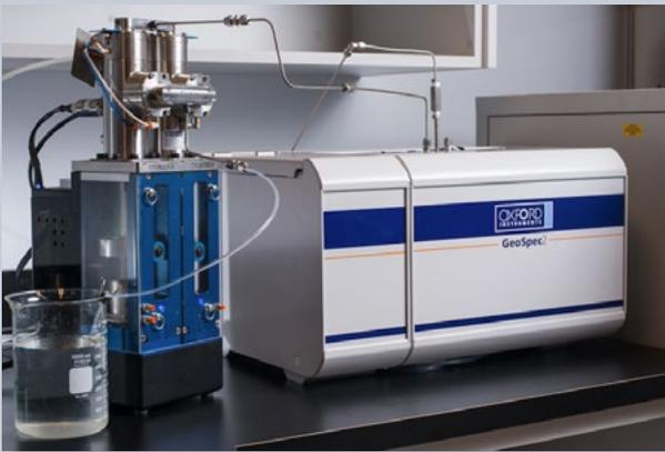
To generate the total gas isotherm, the average total gas content was determined for the shale at 500, 1000, 1500 and 2000 psi. The average was taken from four hours onwards, after the methane content in the rock had stabilized. The resulting total gas isotherm is plotted in Figure 2 (blue trace). The isotherm has the expected curved appearance as a function of pressure, a result of the competing mechanisms of adsorption and absorption.
