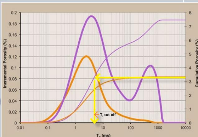
Figure 2 -  $T_2$  distributions showing  $T_2$  cut-off point
