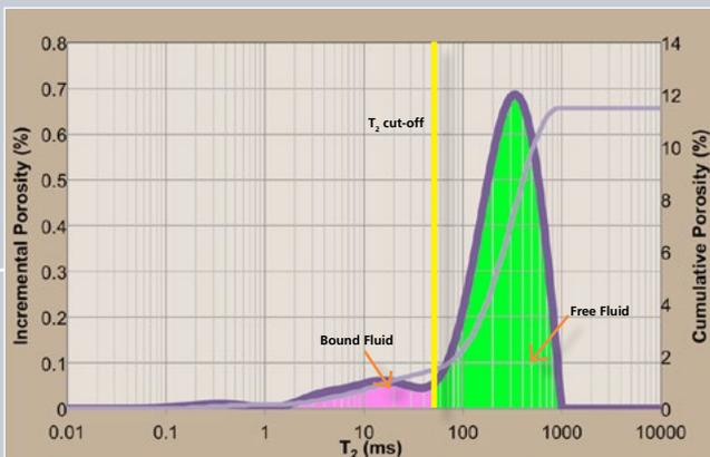
Figure 1 -  $T_2$  distribution showing integral for free fluid
