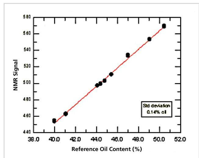
Figure 1: Calibration of oil content of rape seeds in the presence of water (Standard deviation 0.14%)
