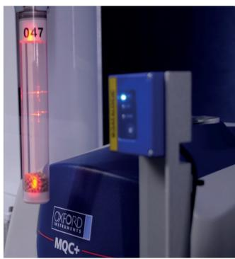
The optional barcode reader records sample ID and recalls previously stored tare weight of the tube.
