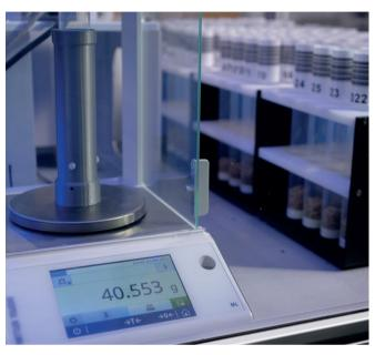
The optional balance automatically records gross weight of sample plus tube.
